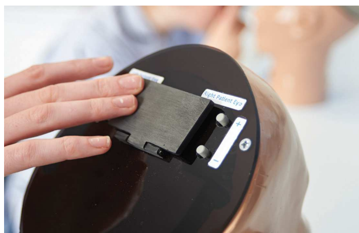
Cover to hide condition LED indicators during examination conditions
